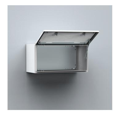
The mild steel single door wall mounted range, MAP, with a IP 66 protection degree, comprises enclosures with a horizontally hinged door plus top and bottom gland plate openings. Each of these enclosures can be easily combined with another wall mounted enclosure, which allows for the creation of configurations with two compartments with individual access.
