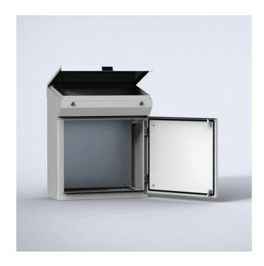
The mild steel compact console, MPG, in a IP 55/56 protection degree is available off the shelf. It has a hinged desk panel, and the ergonomic design allows for easy installation and access to HMI-equipment. It also increases the mounting space available. Stainless steel top panels may be used as an alternative when the console is exposed chemical agents, etc.
