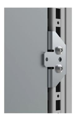
This reinforcement bracket for fitting in the most rear position makes the mounting plate more rigid, which reduces any vibrations, and makes it possible to hold more weight.
