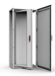
A swing frame for 19" equipment that provides additional mounting space for such equipment, as well as rear access to the fitted components and equipment once opened. It also provides extra space on the lock side of the 19" profiles to optimize the useful depth for equipment to be fixed to the swing frame.
