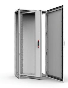
A swing frame for 19" equipment that provides additional mounting space for such equipment, as well as rear access to the fitted components and equipment once opened. It also provides extra space on the lock side of the 19" profiles to optimize the useful depth for equipment to be fixed to the swing frame.
