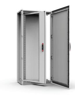
A swing frame for 19" equipment that provides additional mounting space for such equipment, as well as rear access to the fitted components and equipment once opened. It also provides extra space for cabling purposes and increases the useful depth for equipment to be fixed to the swing frame.
