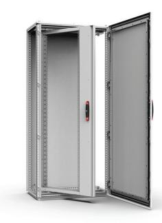
A swing frame for 19" equipment that provides additional mounting space for such equipment, as well as rear access to the fitted components and equipment once opened. It also provides extra space for cabling purposes and increases the useful depth for equipment to be fixed to the swing frame.
